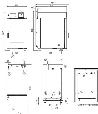
Heat Source: 500mm clearance from an external heat source is required in order to protect the oven control components. For clearances under 500mm, it is mandatory for Stoddart heat shields to be fitted while still maintaining a minimum clearance of 50mm to allow access to the unit. Failure to adhere to minimum clearances may void the oven warranty or add service costs due to lack of access.
